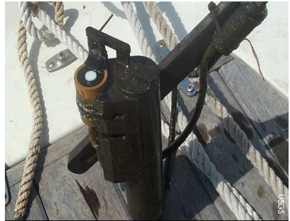
Figure 2. A YSI PAR wiped sensor system prior to deployment
