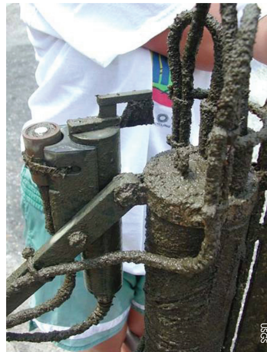
Figure 3. YSI 6600EDS with wiped PAR sensor system after retrieval from deployment. Note the heavy fouling of the sonde in contrast with the clean PAR sensor head.
