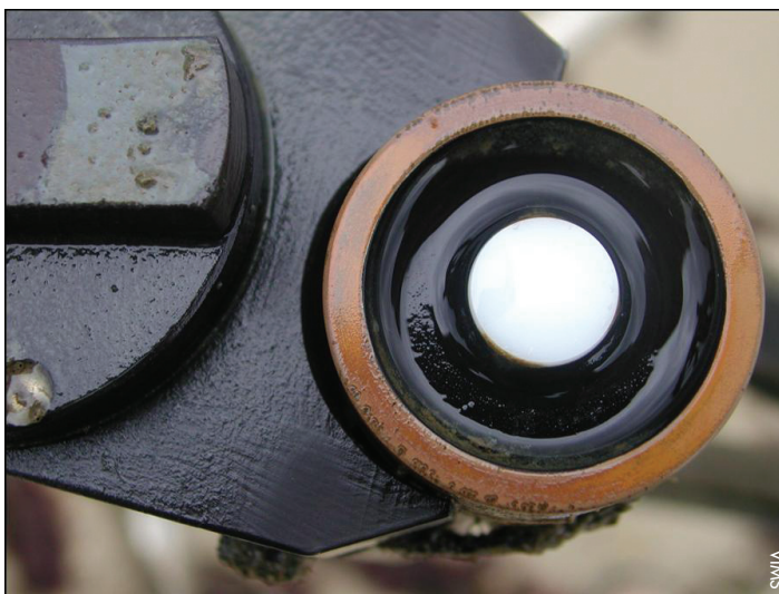
Figure 5. Wiped PAR sensor after 8-day deployment.
