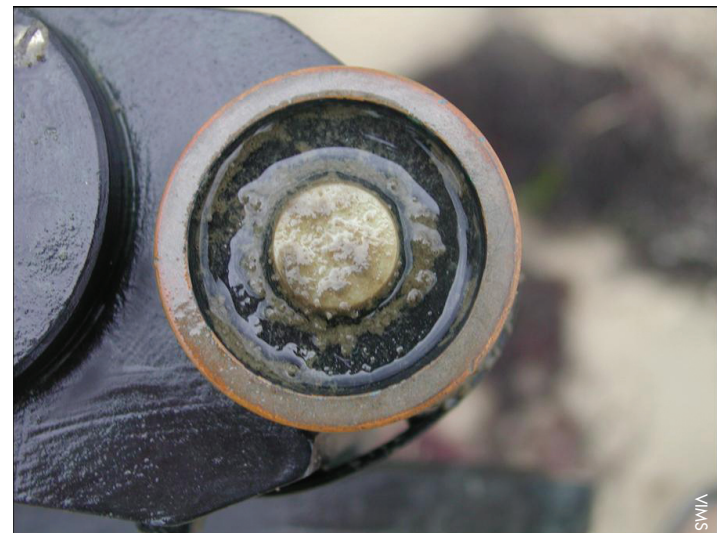
Figure 6. Non-wiped PAR sensor after 8-day deployment.
