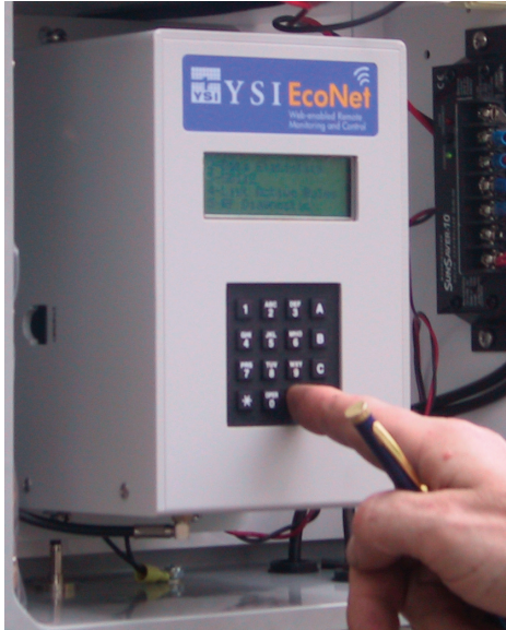
YSI EcoNet Data Node with optional LCD screen and Keypad.
