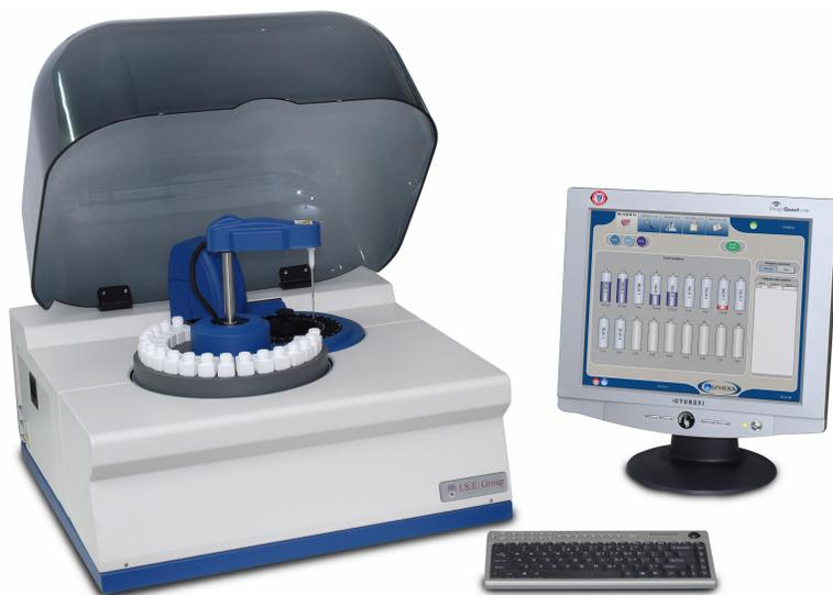
**Random access** automatic analyzer with 60 positions samples tray including blank, controls and calibrants cups.
