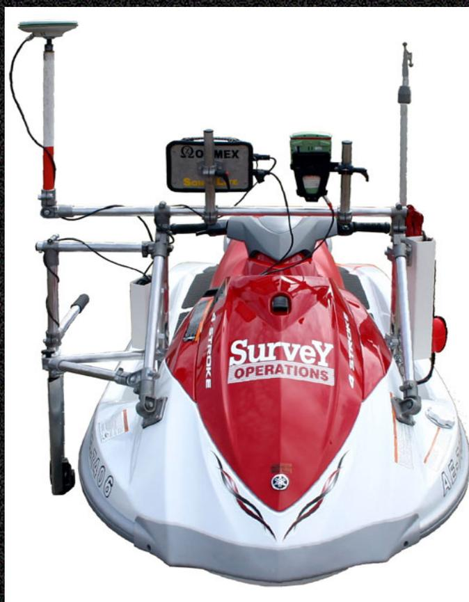
The system comprises a Leica 530 RTK GPS with a SonarLite working in slave mode with its data saved on the Leica control unit.
