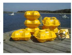
Our steel buoys are depth rated from 380 meters to 564 meters. They are leak tested, anode protected, and coated with a durable epoxy finish. Each sphere includes lifting bails and an internal tension member with pad eyes for convenient and dependable inline use.
