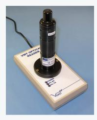
VMT data is stored in the tag memory and can be retrieved using the VMT Optical Reader.
