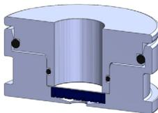
A small array format puck (SAF) is used during the sample processing. A SAF puck is assembled from an SAF top and an SAF bottom. A SAF puck contains a probe array on a nitrocellulose membrane supported by a polysulfone disc. Currently, small format arrays have been designed for phases running the domoic acid (DA) and Saxitoxin (STX) protocols.
