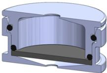
A high-volume sample puck (HVS) is used during sample collection when the environmental occurrence of a target microorganism is low, requiring a larger volume of water to be collected (one to 10 liters). A HVS puck is assembled using a HV2 top and an SH1 bottom, and is loaded with a sintered titanium frit.
