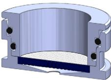
A large array format puck (LAF) is used during sample processing. A LAF puck is assembled from an LAF top and an LAF bottom. A LAF puck contains a probe array on a nitrocellulose membrane supported by a polysulfone disc. Pre-configured arrays have been designed for several algal, bacterial, and larval organisms.
