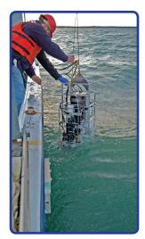
Upper image shows the submersible FlowCAM being deployed from a research vessel. Left image shows remote control and monitoring of the instrument from inside the vessel. Standard VisualSpreadsheet®
